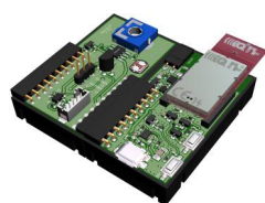
Sensor kit temperature, light intensity and voltage
