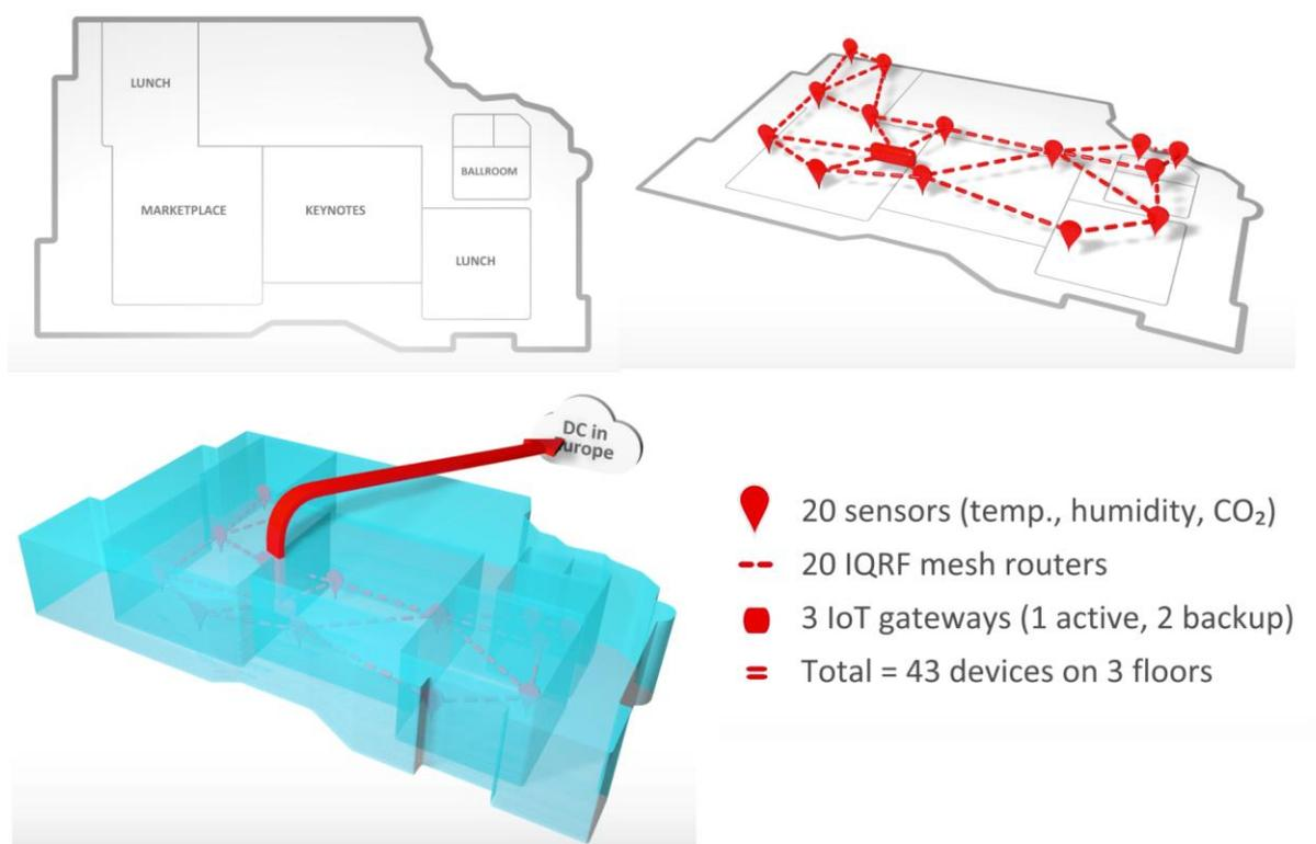
The following picture shows single wireless IQRF mesh network during sensors and routers discovery. Zones 0 - 1 cover conference floor 1 and 2 - 4 floor 4.
