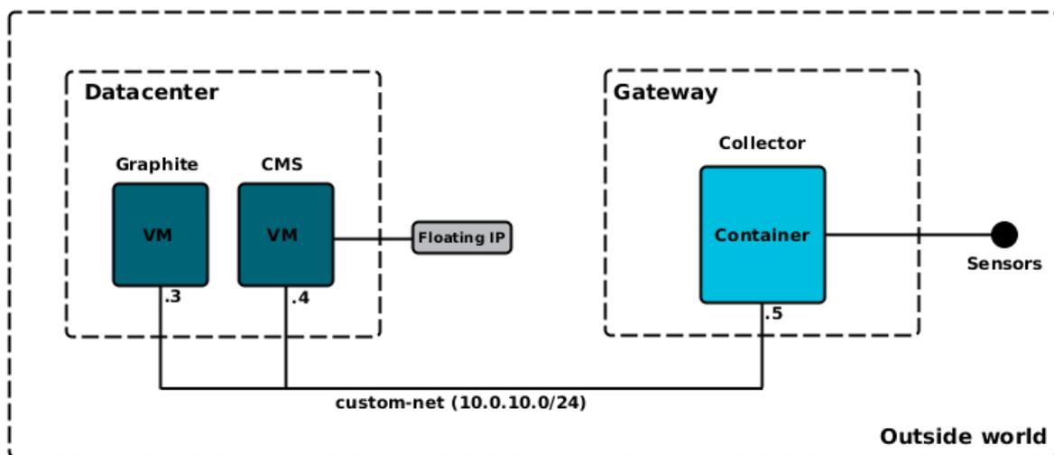
For instance we gather data from environmental sensors. Sensor is directly connected to container where data is processed in Docker container and send them to Graphite time series database. Because we want to present data graphically and realtime we use another VM with Leonardo CMS which reads from Graphite APIs and displays data on website. Accordingly to this we can create different projects on same principles in same cloud with multiple inputs and outputs.
