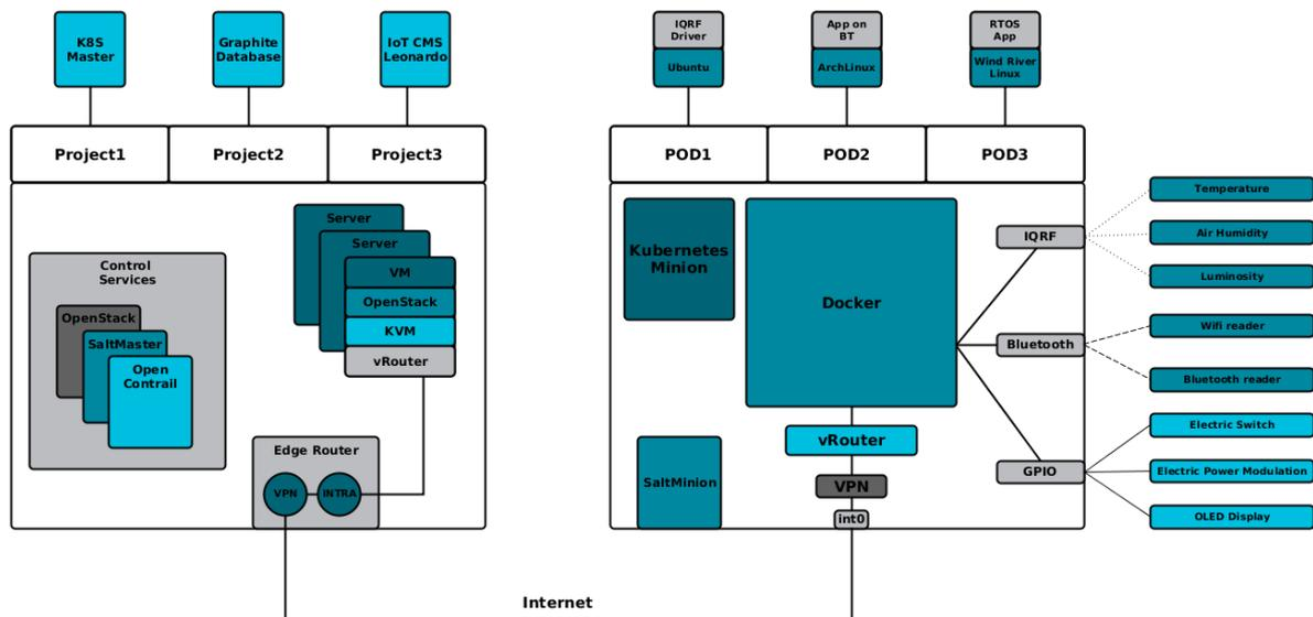
As already mentioned segmentation is done by SDN overlays. The important is only IP connectivity between datacenter edge router and IoT gateway. Lowest layer is VPN between gateway gateway OS and Edge Router in DC. Next layer is SDN, where OpenContrail enables direct communication between VM (OpenStack Cloud) and Container(Gateway). This approach allows to choose from variety of sensors and actuators, privilege them and securely connect with processing applications inside of cloud.
