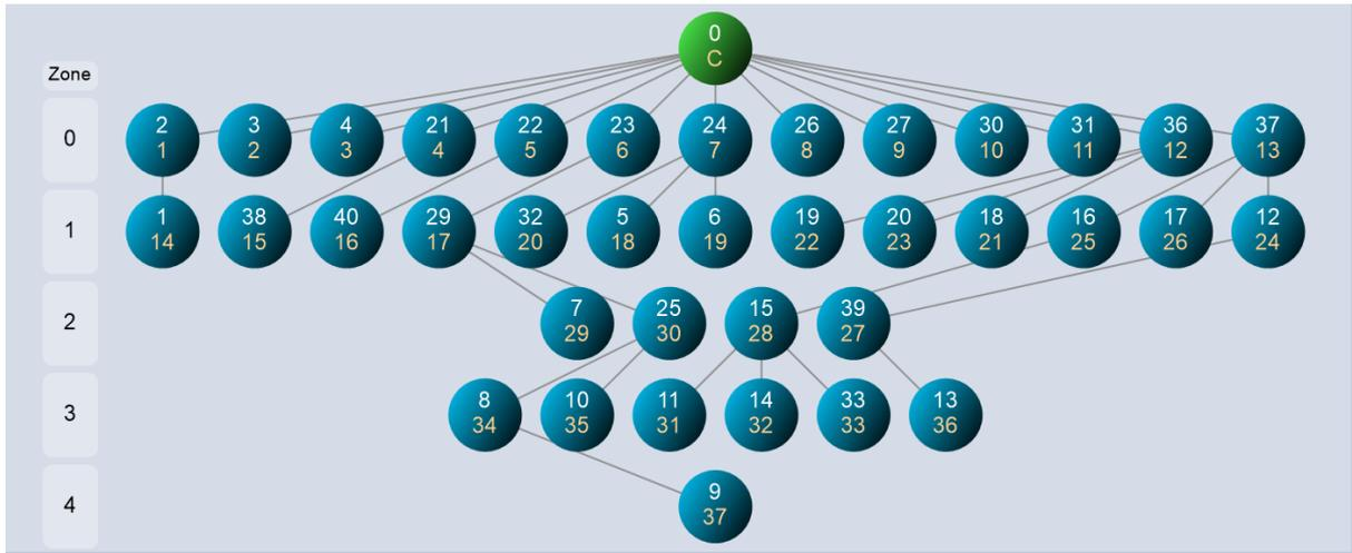
IQRF is a wireless mesh technology operating on sub-gigahertz ISM bands. It provides very easy integration, product interoperability, robust mesh networking with maximum of 240 hops, range of hundreds of meters and ultra-low power operation.
